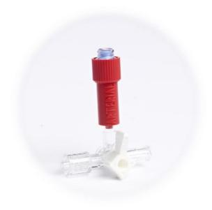
The needle-free non-injectable connector is a device that contains a unique one-way valve mechanism which allows blood sampling but prevents anything else being injected into the arterial line. The design prevents blood from leaking out of the system should the three-way tap be left open.
